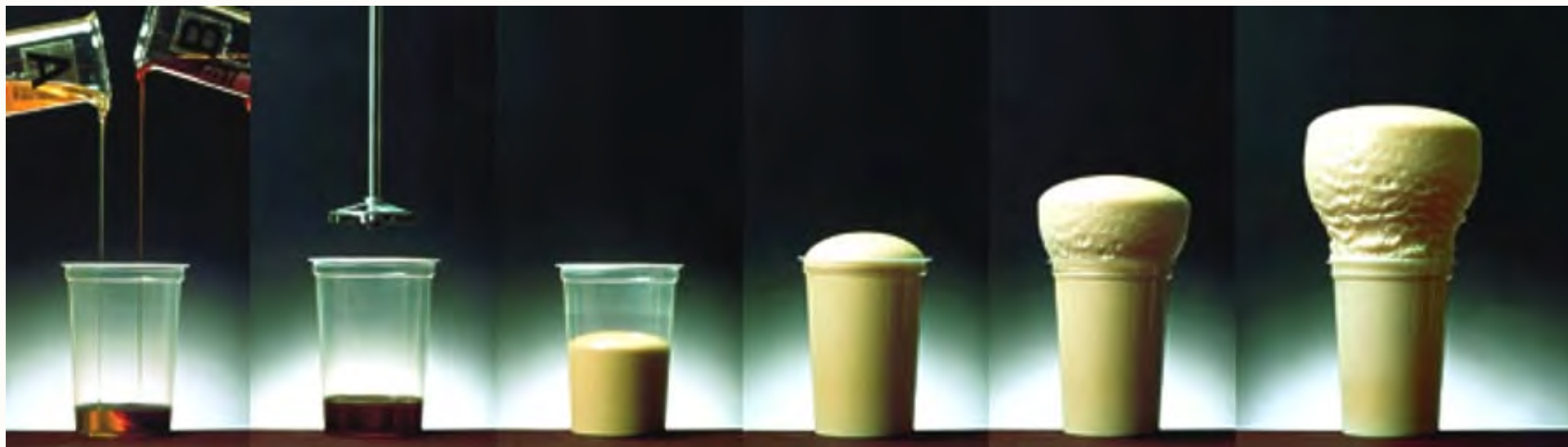
Two-component polyurethane is measured, mixed and poured — expanding into the cushioned foam at the heart of every comfort sole.
